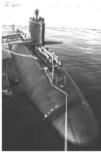
The successful hull-form was applied to the last class of U. S. diesel boats, "Barbel," 1959, (shown here) and to the "Skipjack" nuclear class, 1959.
