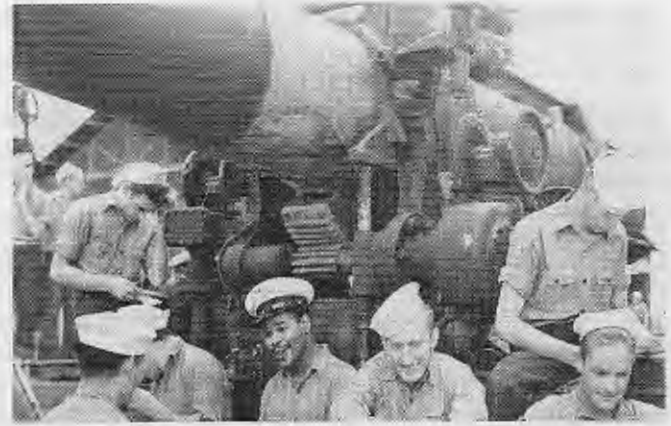
USS V-4 (later Argonaut SS-166, later APS-1) was one of two submarines with large caliber 6"/53 (15.2 cm) deck guns. She had one forward and aft.
